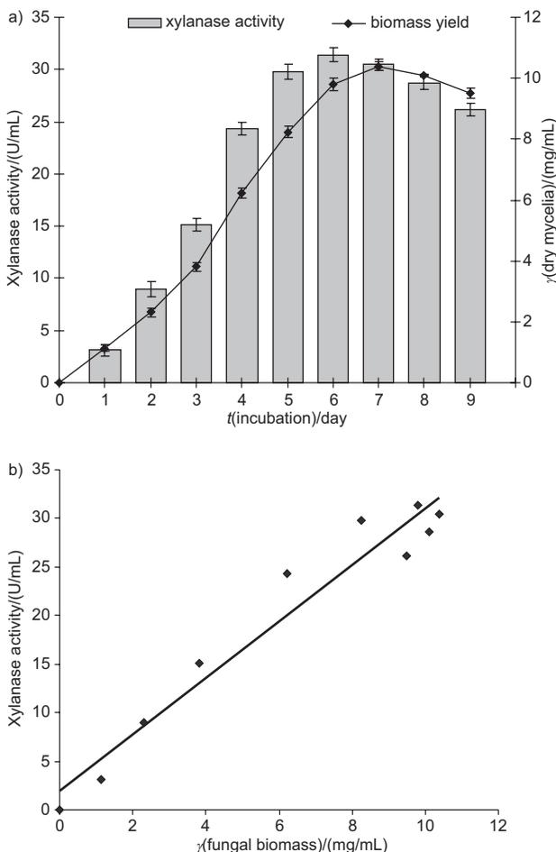
Fig. 6. Xylanase production in an optimized medium: a) effect of fermentation time on growth and xylanase production by *A. flavus* DFR-6, and b) plot between fungal biomass and xylanase activity
