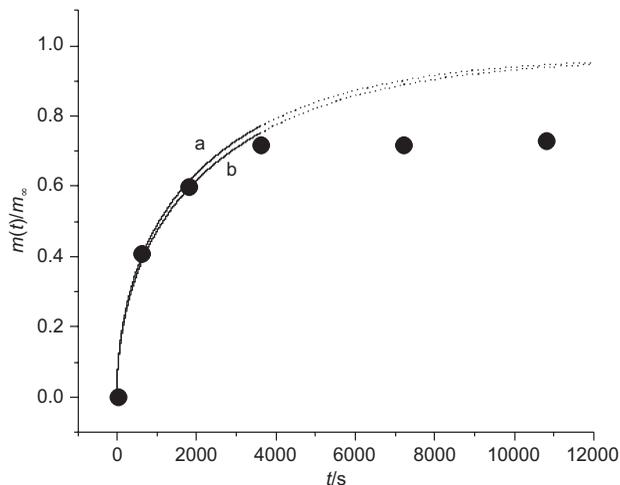
Fig. 7. AA release from xerogel. Dots: experimental results. The lines represent two release curves estimated from Robinson *et al.* (11) using  $D_{\text{eff}}$  values of  $1.90 \cdot 10^{-7}$  and  $1.75 \cdot 10^{-7}\text{ cm}^2/\text{s}$ , respectively
