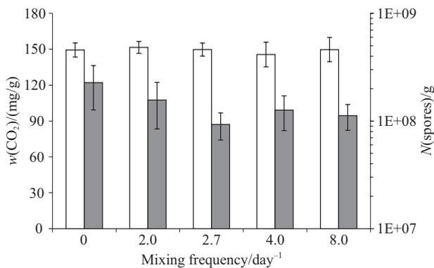
**Fig. 2.** Carbon dioxide (white bars) and spore (grey bars) production at the end of a 48-hour solid-state fermentation of CP by *A. tamarii* V12307 in column reactors using different mixing frequencies
