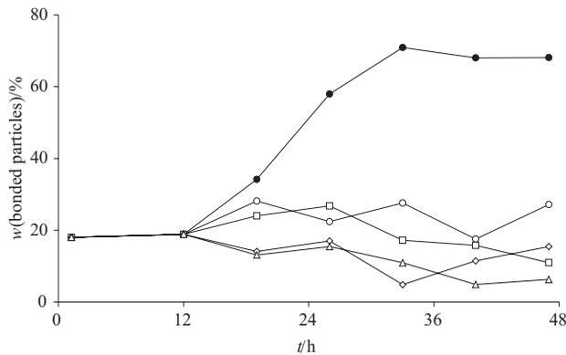
**Fig. 1.** Bonded particle fraction during the solid-state fermentation of coffee pulp by *A. tamarii* V12037 in bottle reactors. After a static period of 12 h, four different daily mixing frequencies were applied: (○) 2.0, (□) 2.7, (◇) 4.0 and (△) 8.0 day<sup>-1</sup>, (●) without mixing
