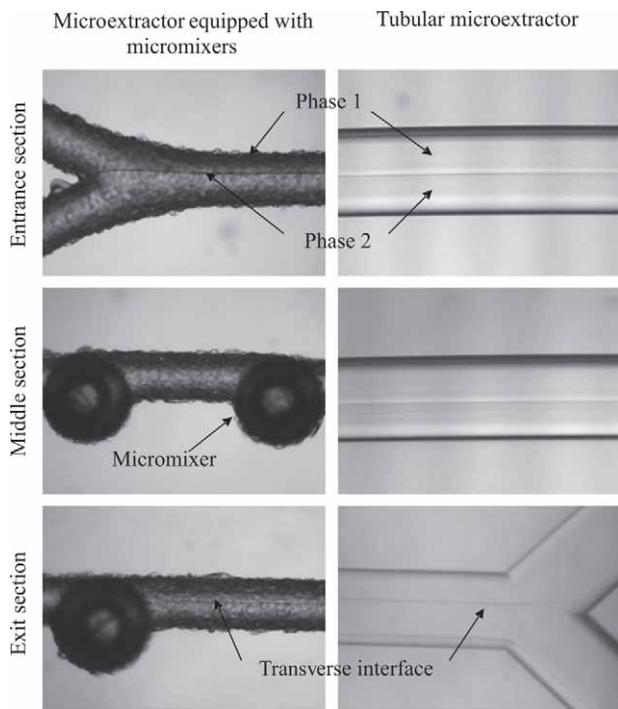
**Fig. 3.** Phase separation at stable laminar flow with the aqueous-aqueous interface formed in the middle of the microchannel at different positions across the microextractor equipped with micromixers and tubular microextractor. Aqueous PEG<sub>6000</sub> solution flow rate of 10  $\mu\text{L}/\text{min}$ , aqueous AMS solution flow rate of 30  $\mu\text{L}/\text{min}$
