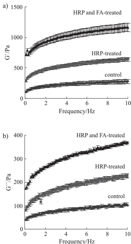
Fig. 5. a) storage modulus ( $G'$ ) and b) loss modulus ( $G''$ ) of the yoghurt samples prepared from the skimmed milk (control) and skimmed milk treated with HRP only, or with HRP and FA and stored at 4 °C for 36 h
