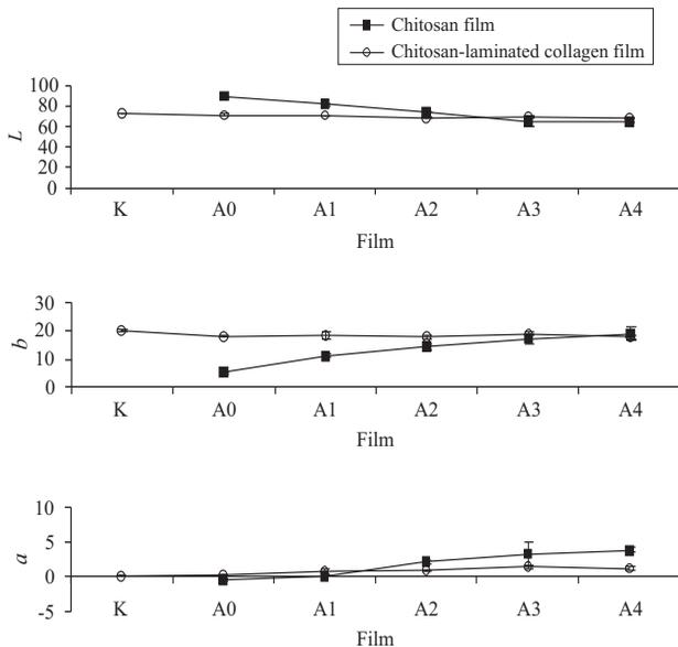
Fig. 9. Film colour parameters ( $L$ ,  $a$  and  $b$  values) of chitosan and chitosan-laminated collagen films. Bars represent the mean values  $\pm$  S.D. of 5 independent measurements. For film labels see Table 1
