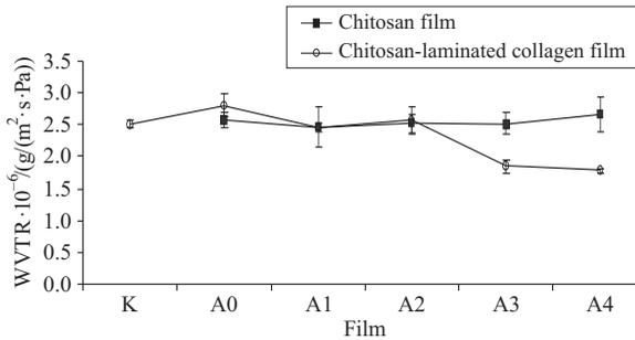
Fig. 6. Water vapour transmission rate (WVTR) of chitosan and chitosan-laminated collagen films. Bars represent the mean values  $\pm$ S.D. of 5 independent measurements. For film labels see Table 1
