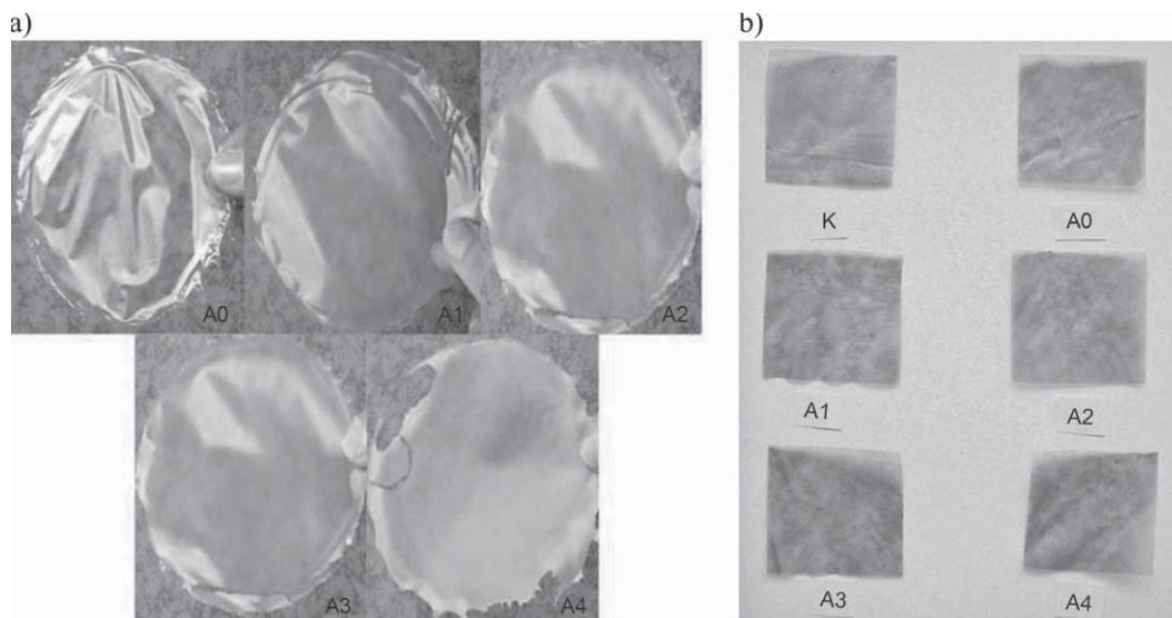
**Fig. 1.** Photographs showing the effect of the addition of different volumes of oregano essential oil (OEO): a) samples of chitosan films, b) samples of collagen film and chitosan-laminated collagen films. For film labels see Table 1
