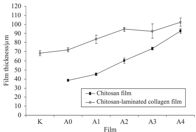
**Fig. 2.** Thickness of chitosan and chitosan-laminated collagen films. Bars represent the mean values±S.D. of 15 independent measurements. For film labels see Table 1
