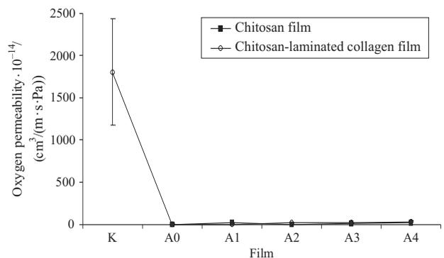
Fig. 8. Oxygen permeability of chitosan and chitosan-laminated collagen films. Bars represent the mean values  $\pm$ S.D. of 5 independent measurements. For film labels see Table 1
