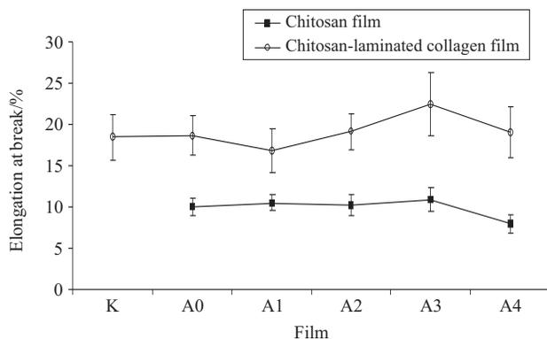
**Fig. 4.** Elongation at break of chitosan and chitosan-laminated collagen films. Bars represent the mean values $\pm$ S.D. of 15 independent measurements. For film labels see Table 1
