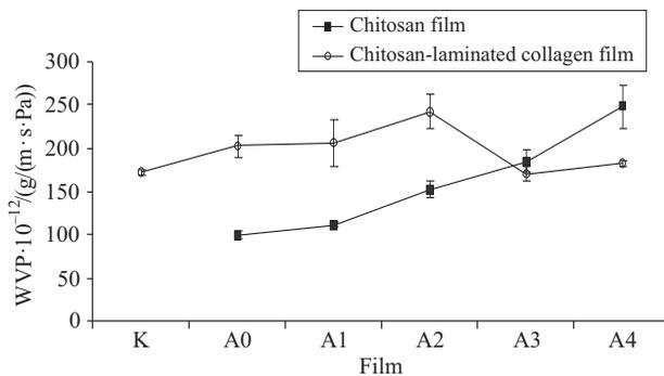
Fig. 7. Water vapour permeability (WVP) of chitosan and chitosan-laminated collagen films. Bars represent the mean values  $\pm$ S.D. of 5 independent measurements. For film labels see Table 1
