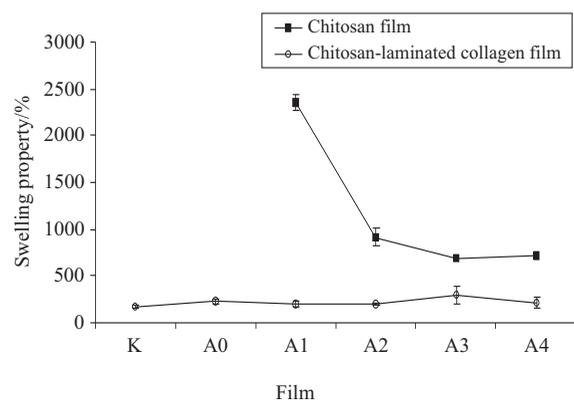
**Fig. 5.** Swelling property of chitosan and chitosan-laminated collagen films. Bars represent the mean values $\pm$ S.D. of 5 independent measurements. For film labels see Table 1
