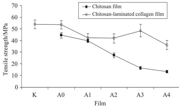
**Fig. 3.** Tensile strength of chitosan and chitosan-laminated collagen films. Bars represent the mean values $\pm$ S.D. of 15 independent measurements. For film labels see Table 1
