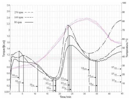
**Fig. 2.** Mixolab curves recorded at different mixing speeds (80, 160 and 250 rpm) for good quality baking flour S1=initial mixing, S2=protein weakening, S3=starch gelatinization, S4=stability during baking, and S5=retrogradation are the stages of Mixolab curves; pink curves indicate dough temperature
