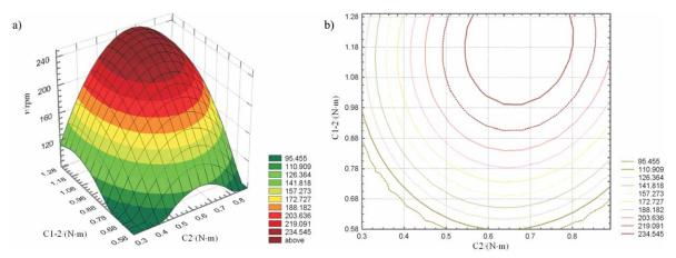
Fig. 5. Mixing speed (v) as a function of torque for the minimum consistency in the second stage of the curve (C2), and difference between points C1 and C2 (C1-2): a) spatial representation, and b) representation by contour curves
