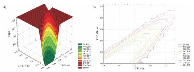
**Fig. 6.** Mixing speed (*v*) as a function of torque for the maximum consistency in the third stage of the curve (C3), and difference between points C3 and C2 (C3-2): a) spatial representation, and b) representation by contour curves
