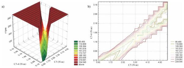
**Fig. 8.** Mixing speed (*v*) as a function of torque for the maximum consistency in the fifth stage of the curve (C5), and difference between points C5 and C4 (C5-4): a) spatial representation, and b) representation by contour curves
