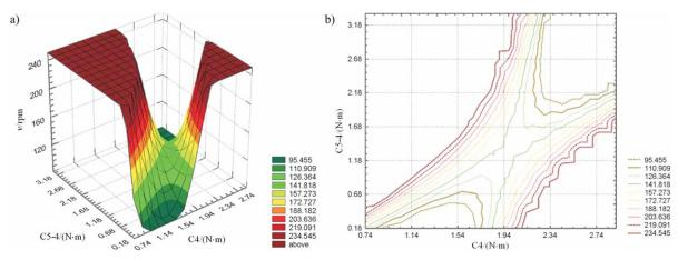
Fig. 7. Mixing speed (v) as a function of torque for the minimum consistency in the fourth stage of the curve (C4), and difference between points C5 and C4 (C5-4): a) spatial representation, and b) representation by contour curves
