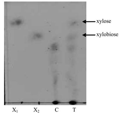
**Fig. 8.** Time course of wheat bran hydrolysis by the recombinant xylanase. Wheat bran was incubated at 60 °C with 20 U/mL of XynBT21 for 24 h and analysed by thin-layer chromatography. Xylose ( $X_1$ ) and xylobiose ( $X_2$ ) are standards, while C is control (sample without enzyme fraction) and T is the test sample with active enzyme
