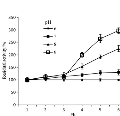
Fig. 3. Effect of pH on xylanase stability. The enzyme was diluted with phosphate buffers of various pH values and incubated at room temperature for  $t=24$  h. Residual activity was assayed at pH=6 and 60 °C
