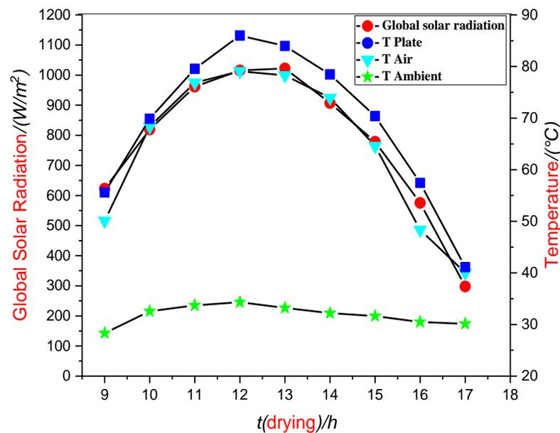
Fig. S2. Variation of solar radiation, ambient temperature, drying air temperature, absorber plate temperature with the drying time of the samples: a) natural convection dryer, b) forced convection dryer
