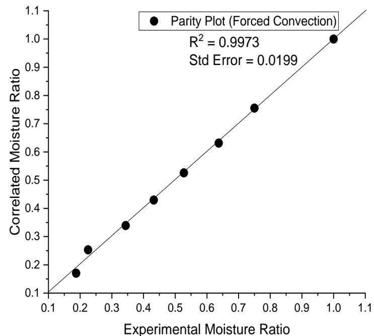
Fig. S3. Parity plot for experimental moisture ratio vs correlated moisture ratio: a) natural convection dryer, b) forced convection dryer
