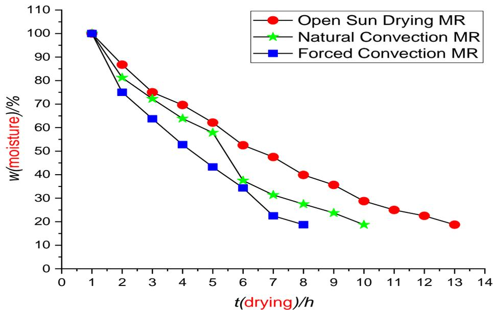
Fig. 1. Variation of moisture ratio of the samples with the drying time for open, natural and forced solar drying
