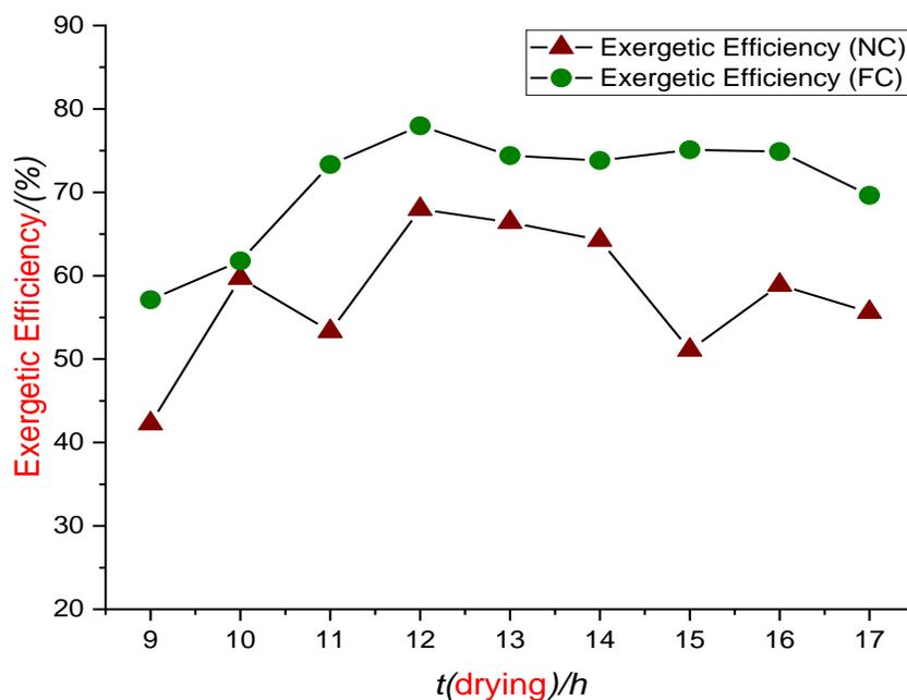
Fig. 4. Variation of exergetic efficiency with the drying time of the samples
