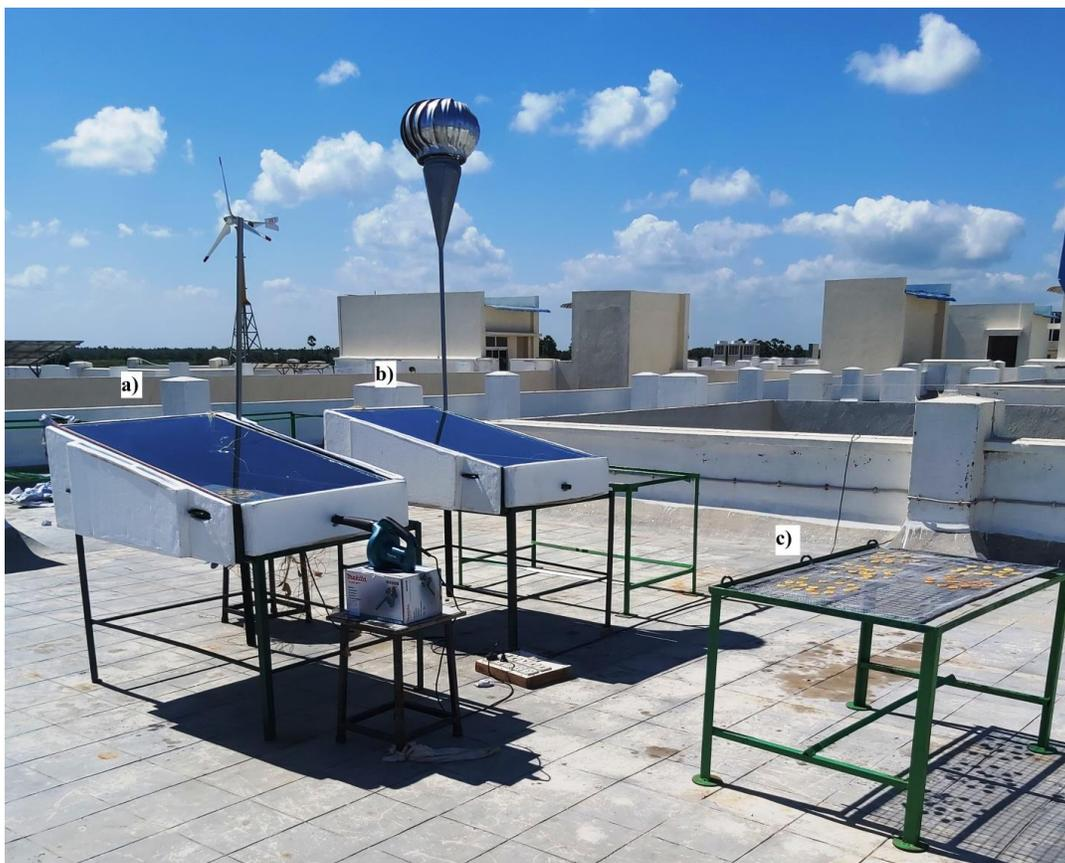
**Fig. S1.** Photograph of experimental setup of banana drying: a) natural convection, b) forced convection single slope solar dryer and c) open sun drying
