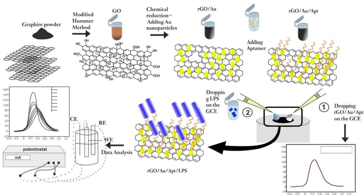
**Fig. 4.** schematic of electrochemical aptasensing of lipopolysaccharides from *Escherichia coli* bacteria. Reproduced from Ref. (5) with permission
