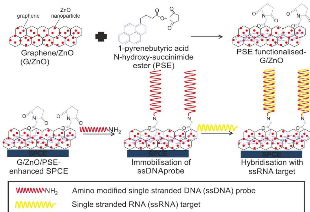
**Fig. 3.** Schematic diagram for the development of graphene/zinc oxide nanocomposite-modified electrochemical impedance genosensor for ssRNA detection, Reproduced from Ref. (38) with permission
