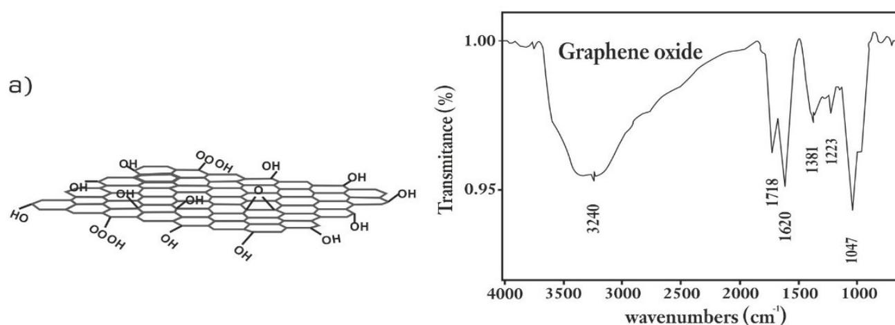
**Fig. 3.** Structure of GO (left) and its FTIR spectrum (right). Reproduced from Ref. (1) with permission
