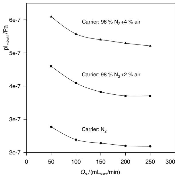
Fig. 5. Effect of carrier gas composition and flow rate on the MS response at a mass to charge ratio  $m/z=32$  at a constant flow rate of 148 mL/min of water saturated with oxygen
