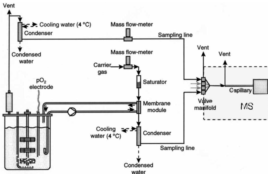
Fig. 2. Experimental set-up for testing module and for the optimisation of the operating conditions
