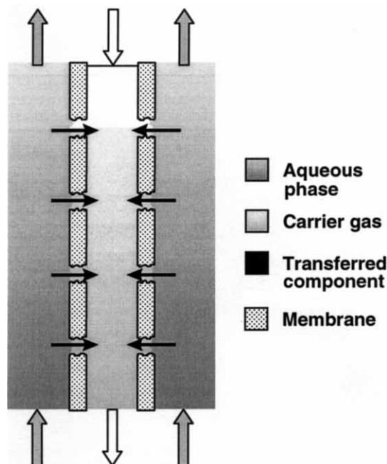
Fig. 1. Operating scheme of the microporous hydrophobic hollow fibre module
