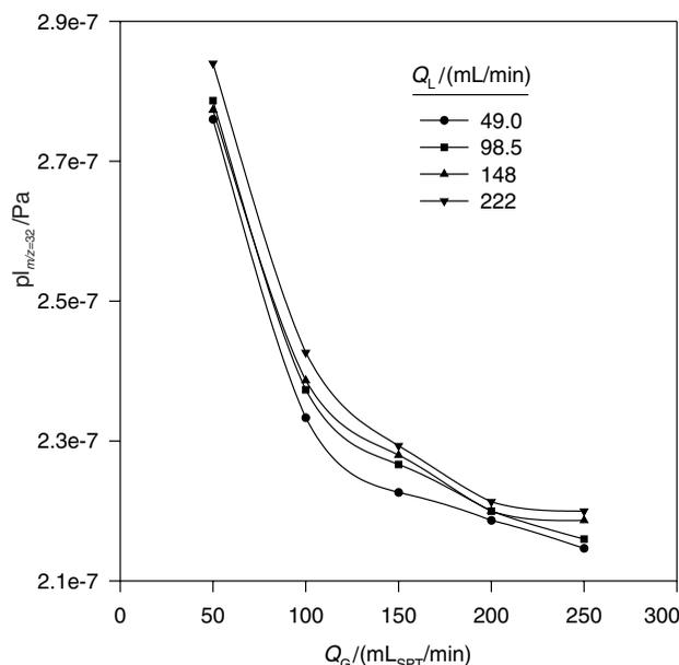
Fig. 4. Effect of the flow rates of the carrier gas (nitrogen),  $Q_G$ , and of the recirculated water saturated with oxygen,  $Q_L$ , on the MS response at a mass to charge ratio  $m/z=32$
