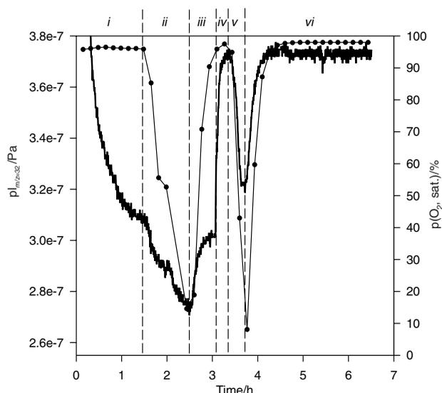
Fig. 3. MS measurements of dissolved oxygen (—) compared with measurements obtained with an oxygen electrode (●)
