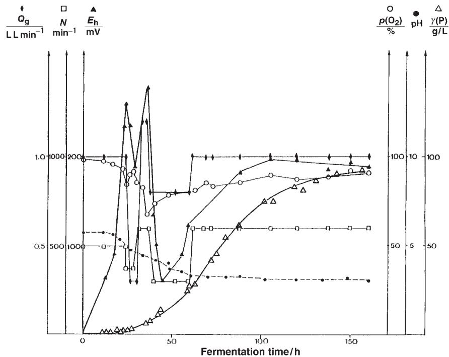
Fig. 7. Process parameters of citric acid yielding bioprocessing at physical regulation;  $\blacktriangle$   $E_h$  redox potential,  $\circ$   $p(O_2)$ , dissolved oxygen partial pressure,  $\blacklozenge$   $Q_g$  aeration rate,  $\square$   $N$  impeller speed,  $\triangle$   $P$  citric acid
