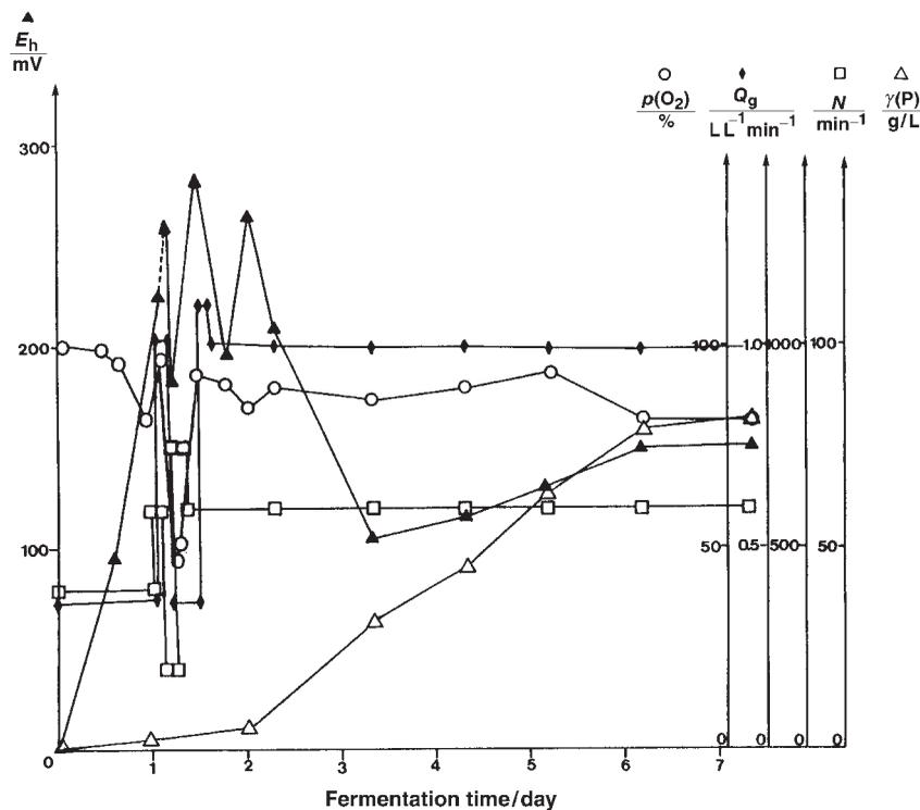
Fig. 5. Process parameters of citric acid yielding bioprocessing at physical regulation; ▲  $E_h$ , redox potential, ○  $p(O_2)$ , dissolved oxygen partial pressure, ◆  $Q_g$  aeration rate, ◻  $N$  impeller speed, △  $P$  citric acid
