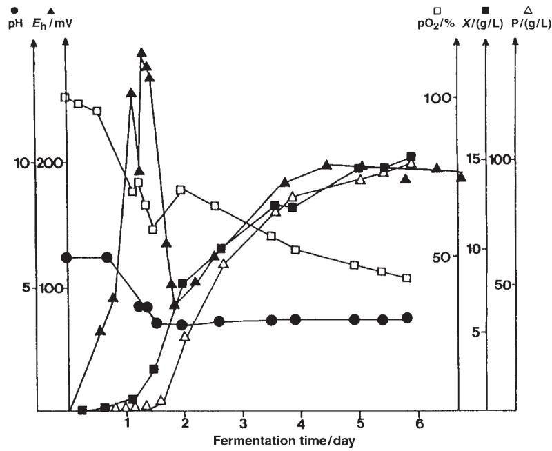
Fig. 1. Process parameters of high citric acid yielding bioprocessing; ▲ E<sub>h</sub> redox potential, □ p(O<sub>2</sub>) dissolved oxygen partial pressure, ● pH, ■ X biomass, Δ P citric acid
