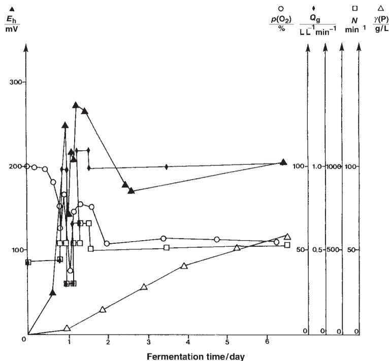
Fig. 6. Process parameters of citric acid yielding bioprocessing at physical regulation;  $\blacktriangle$   $E_h$ , redox potential,  $\circ$   $p(O_2)$ , dissolved oxygen partial pressure,  $\blacklozenge$   $Q_g$  aeration rate,  $\square$   $N$  impeller speed,  $\triangle$   $P$  citric acid
