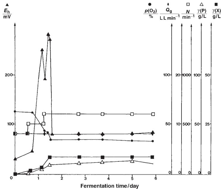
Fig. 2. Process parameters of citric acid bioprocessing at chemical regulation of redox potential using 0.1 % sodium sulphite as reductant and 0.1 % hydrogen peroxide as oxidant; ▲ E<sub>h</sub> redox potential, ● p(O<sub>2</sub>) dissolved oxygen partial pressure, ■ X biomass, Δ P citric acid, ◆ Q<sub>g</sub> aeration rate, □ N impeller speed
