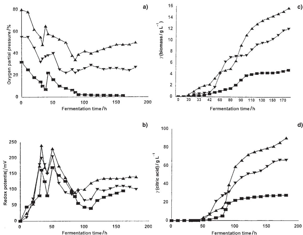
Fig. 4. Oxygen partial pressure (a), redox potential (b), biomass (c) and citric acid (d) time courses at aeration rates  $Q_g$  and impeller speed  $N$ ;  $\blacksquare$   $Q_g = 0.4 L L^{-1} min^{-1}, N = 300 min^{-1}$ ;  $\blacktriangledown$   $Q_g = 0.6 L L^{-1} min^{-1}, N = 500 min^{-1}$ ;  $\blacktriangle$   $Q_g = 1.0 L L^{-1} min^{-1}, N = 700 min^{-1}$
