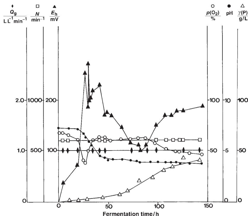
Fig. 3. Process parameters of citric acid bioprocessing at chemical regulation of redox potential using 20 % glucose as reductant and 0.1 % hydrogen peroxide as oxidant;  $\blacktriangle$   $E_h$  redox potential,  $\circ$   $p(O_2)$  dissolved oxygen partial pressure,  $\diamond$   $Q_g$  aeration rate,  $\square$   $N$  impeller speed,  $\Delta$   $P$  citric acid,  $\bullet$  pH
