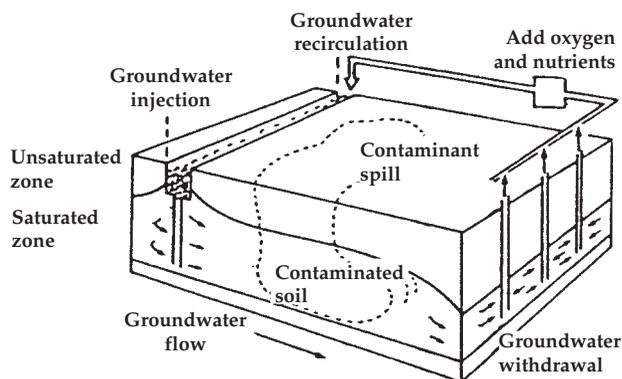
Fig. 1. Schematics of the *in situ* treatment of contaminated saturated soil
