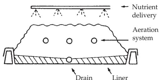
Fig. 3. On-site treatment method for excavated contaminated soil
