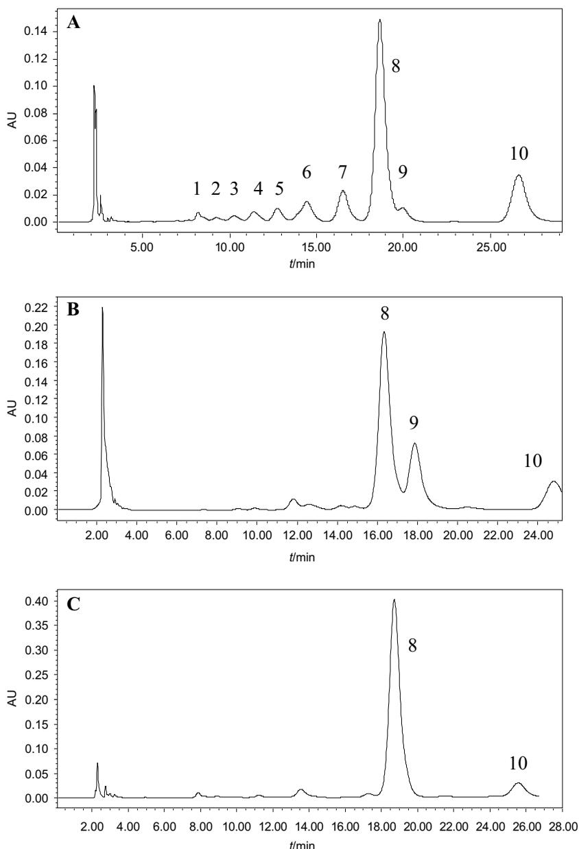
**Fig. 3.** HPLC separation of three kinds of hydrolysates degraded under optimal conditions for agaro-oligosaccharides. (A) Solid acid degradation (70 °C, 10 % of solid acid, 2 % of agar for 8 h). Peaks of oligosaccharides: 1, DP=16; 2, DP=14; 3, DP=12; 4, DP=10; 5, DP=8; 6, DP=6; 7, DP=4; 8, DP=2; 9, monosaccharide; 10,  $\alpha$ -naphthylamine; (B) Citric acid degradation (90 °C, 0.5 M citric acid, 2 % of agar for 3.5 h); (C) HCl degradation (80 °C, 0.37 M HCl, 2 % of agar for 5 h)
