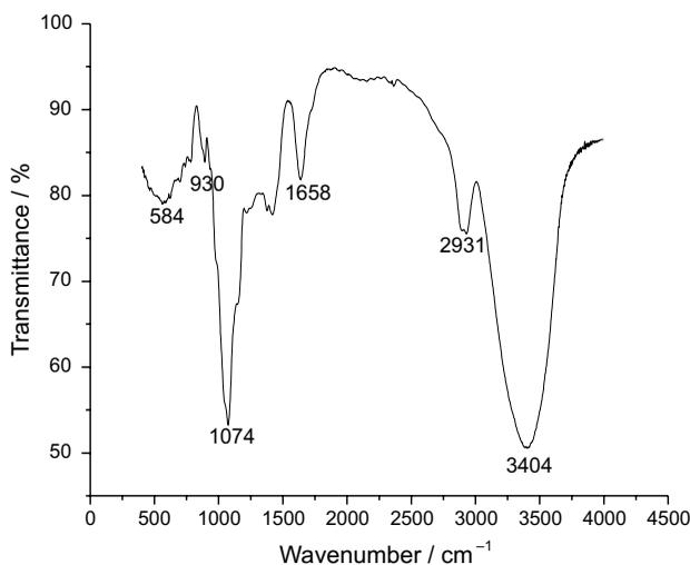
Fig. 1. The FTIR spectrum of solid acid hydrolysate
