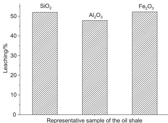
Fig. 2. Percentage of leaching of silicon oxide (SiO<sub>2</sub>), aluminium oxide (Al<sub>2</sub>O<sub>3</sub>) and iron(III) oxide (Fe<sub>2</sub>O<sub>3</sub>) of representative sample of the oil shale
