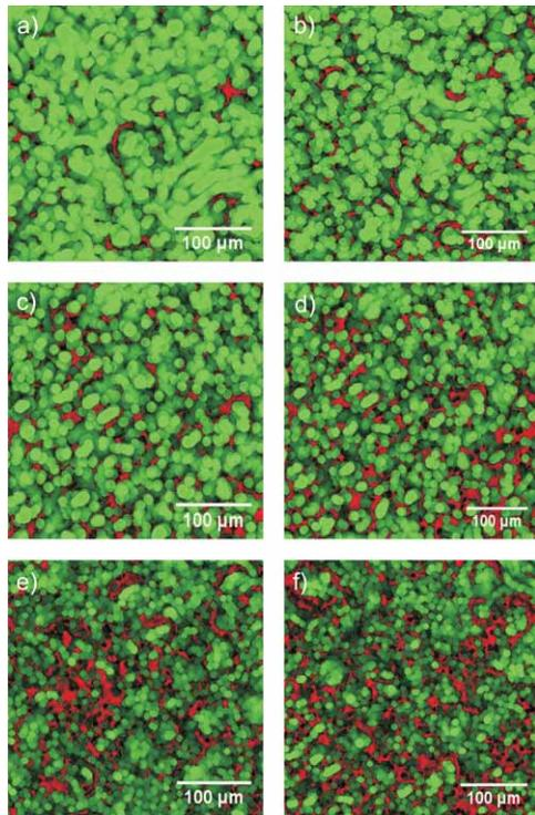
**Fig. 1.** Images of dough microstructure taken by EFLM: a) at 80 rpm for 3 min (5.01 (W·h)/kg), b) at 80 rpm for 5 min (8.70 (W·h)/kg), c) at 160 rpm for 3 min (10.78 (W·h)/kg), d) at 160 rpm for 5 min (18.73 (W·h)/kg), e) at 250 rpm for 3 min (19.96 (W·h)/kg), and f) at 250 rpm for 5 min (34.81 (W·h)/kg). Green are starch granules, while red is protein
