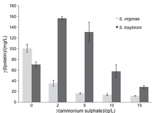
Fig. 6. The effect of ammonium sulphate supplementation in production medium, containing 4 % of soya bean meal and 5 % of soya bean oil, on lipstatin production by *Streptomyces virginiae* and *S. toxytricini* strains
