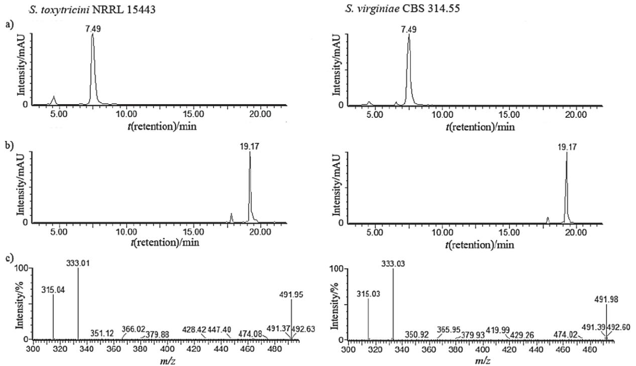
**Fig. 3.** LC-MS/MS analysis of *Streptomyces toxycitricini* NRRL 15443 and *Streptomyces virginiae* CBS 314.55 culture broths compared under different chromatographic conditions: a) gradient starting with 80 % acetonitrile in the mobile phase, b) gradient starting with 50 % acetonitrile in the mobile phase, and c) MS fragment pattern of lipstatin peak at 7.49 min
