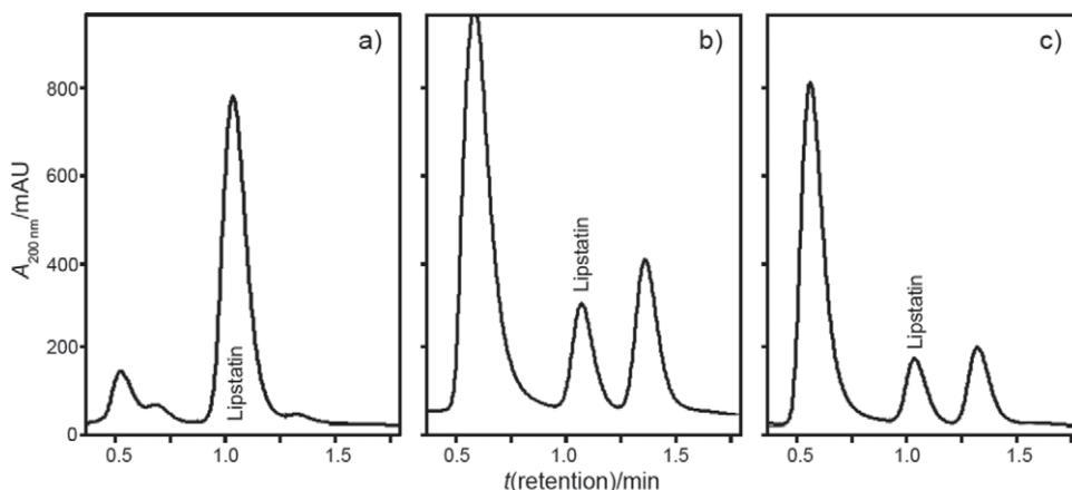
Fig. 2. HPLC analysis of: a) commercial lipstatin standard, and fermentation broth of: b) *Streptomyces toxytricini* NRRL 15443 and c) *Streptomyces virginiae* CBS 314.55 confirms the presence of lipstatin in the fermentation broth of *S. virginiae* AU=arbitrary units
