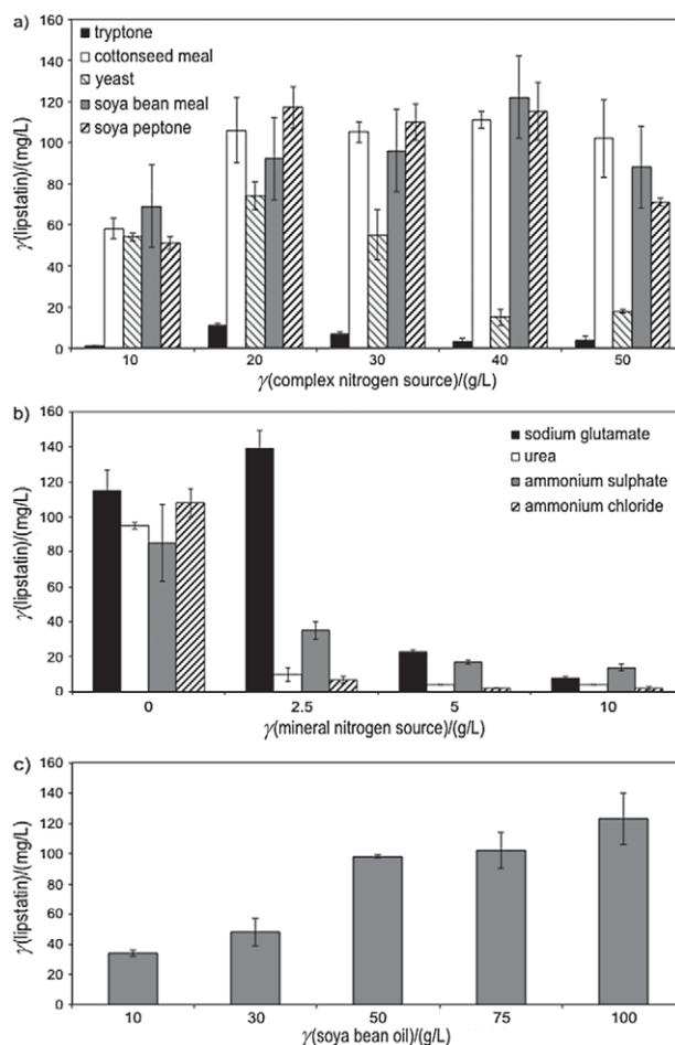
Fig. 5. The effect of carbon and nitrogen sources in the medium on lipstatin production by *Streptomyces virginiae*: a) complex nitrogen sources using fermentation medium with 5 % of soya bean oil, b) supplementation with simple/mineral nitrogen sources using fermentation medium containing 4 % of soya bean meal and 5 % of soya bean oil, and c) effect of the addition of different concentrations of soya bean oil. Error bars present standard deviation from two independent biological replicates
