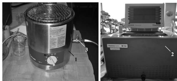
Fig. 1. Experimental set-up (1=ultrasonic bath, 2=temperature-controlled circulating water bath, 3=ball valve)
